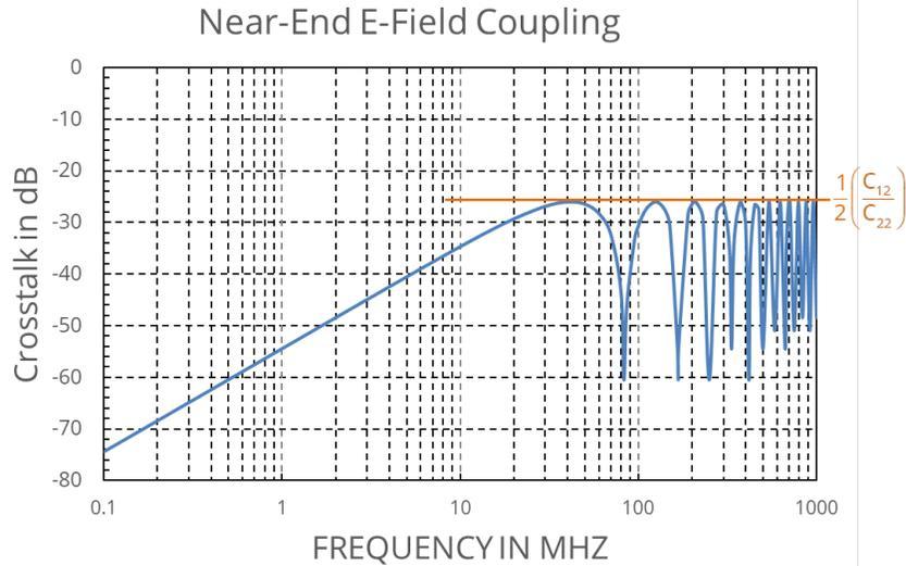
**Figure 6.8.** Near-end crosstalk between two matched transmission lines due to E-field coupling.
