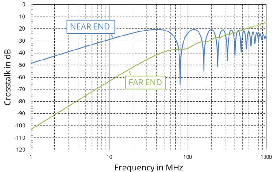
**Figure 6.19.** Calculated crosstalk between two lines with  $C_{12}/C_{22} = L_{12}/L_{11} = 10^{-1}$ .
