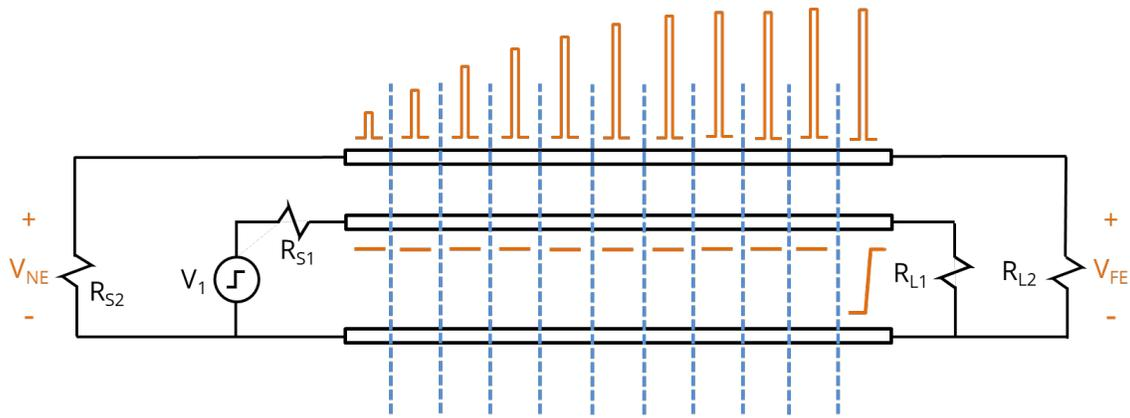
**Figure 6.14.** Crosstalk as the voltage transition reaches the end of the line.
