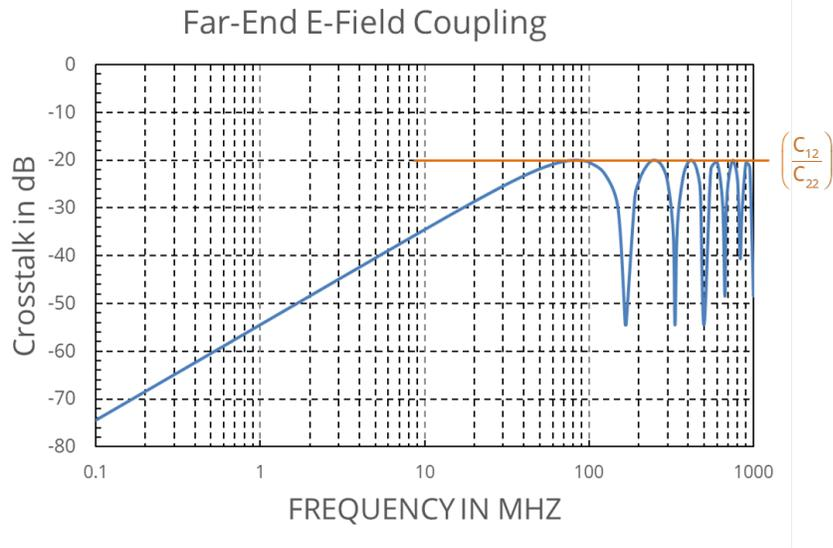
**Figure 6.7.** Far-end crosstalk between two matched transmission lines due to E-field coupling.
