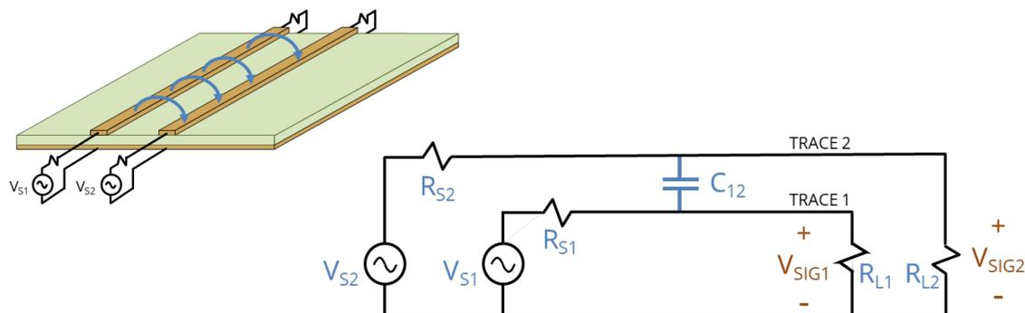
**Figure 6.3.** Schematic representation of electric-field coupling between traces.
