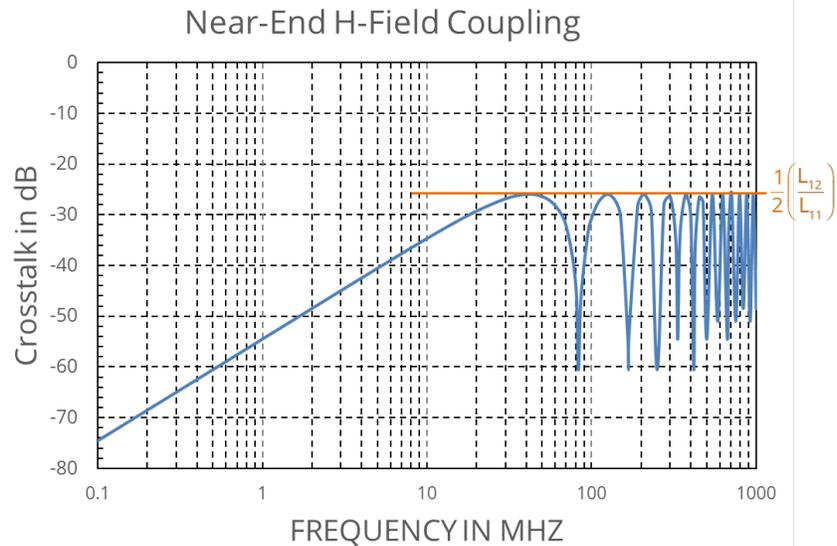
**Figure 6.10.** Near-end crosstalk between two matched transmission lines due to H-field coupling.
