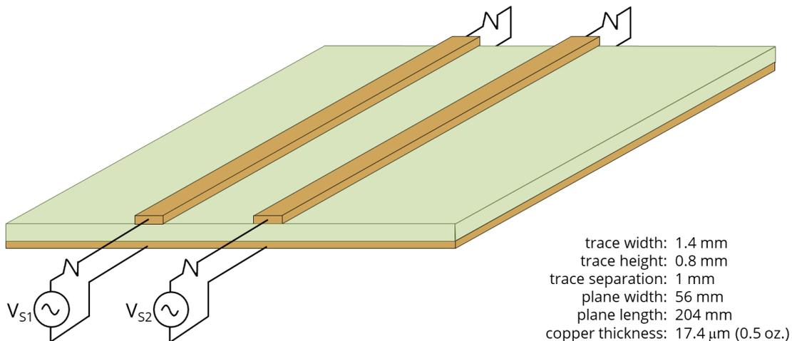
**Figure 6.1.** Two signal traces sharing a circuit board return plane.
