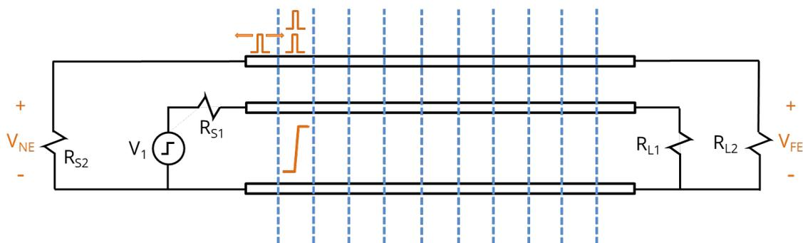
**Figure 6.13.** Crosstalk as the voltage transition begins to move down the line.
