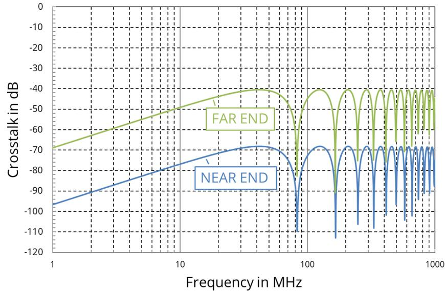
**Figure 6.20.** Calculated crosstalk with  $C_{12}/C_{22} = L_{12}/L_{11} = 10^{-2}$  and  $R_{NE2}=1 \Omega$ .
