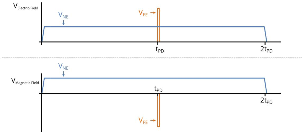
**Figure 6.15.** Near-end and far-end crosstalk for electric- and magnetic-field coupling.
