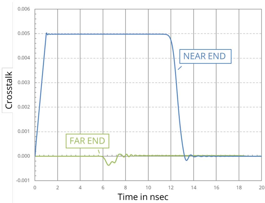
**Figure 6.23.** Calculated crosstalk between matched lines with  $C_{12}/C_{22} = L_{12}/L_{11} = 10^{-2}$ .
