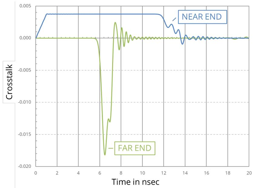
**Figure 6.26.** Calculated crosstalk between matched lines in a non-homogeneous dielectric.
