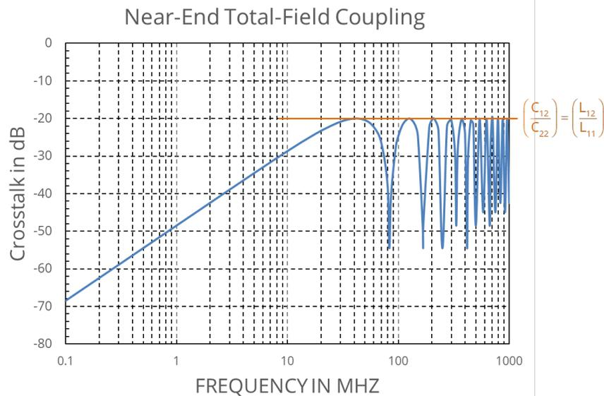
**Figure 6.11.** Total near-end crosstalk between two matched transmission lines.
