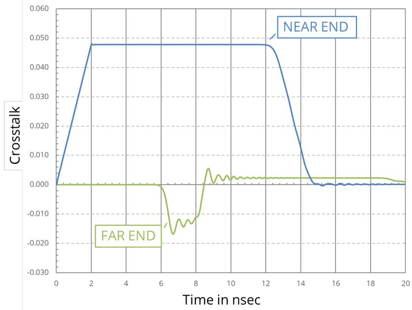
**Figure 6.25.** Calculated crosstalk between matched lines with  $C_{12}/C_{22} = L_{12}/L_{11} = 10^{-1}$ .
