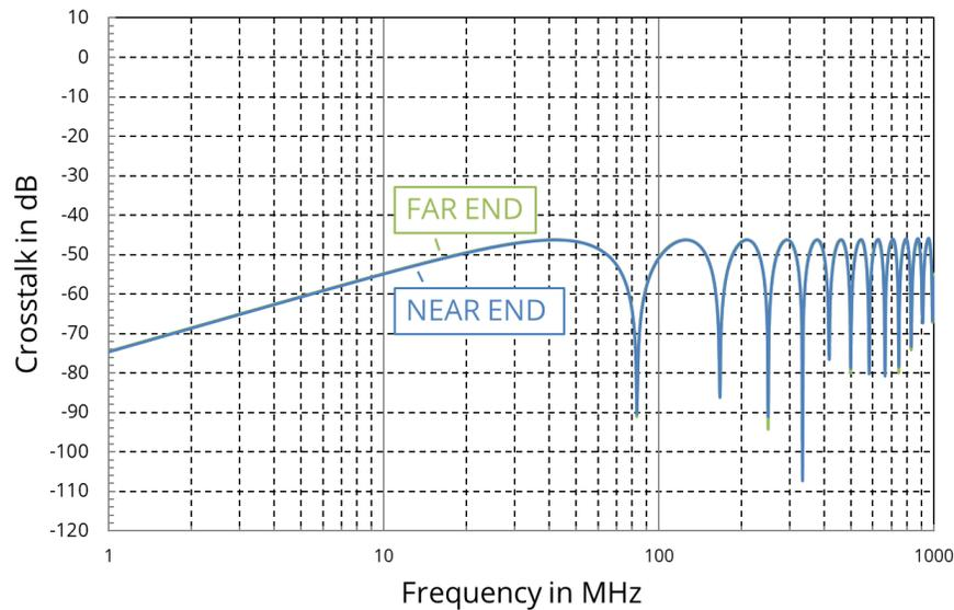
**Figure 6.21.** Calculated crosstalk with  $C_{12}/C_{22} = L_{12}/L_{11} = 10^{-2}$  and  $R_{FE1}=5000 \Omega$ .
