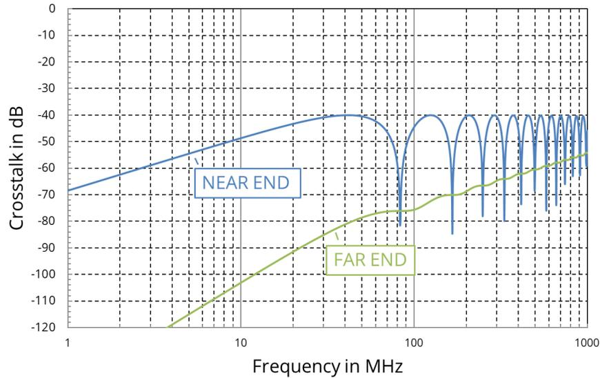
**Figure 6.18.** Calculated crosstalk between two lines with  $C_{12}/C_{22} = L_{12}/L_{11} = 10^{-2}$ .
