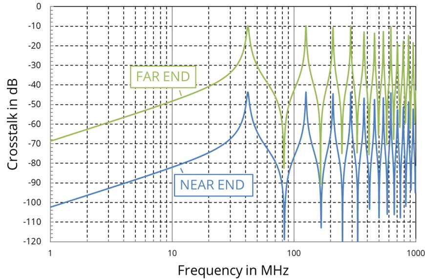
**Figure 6.22.** Calculated crosstalk with  $C_{12}/C_{22} = L_{12}/L_{11} = 10^{-2}$  and  $R_{NE2}=1 \Omega$  and  $R_{FE2}=5000 \Omega$ .
