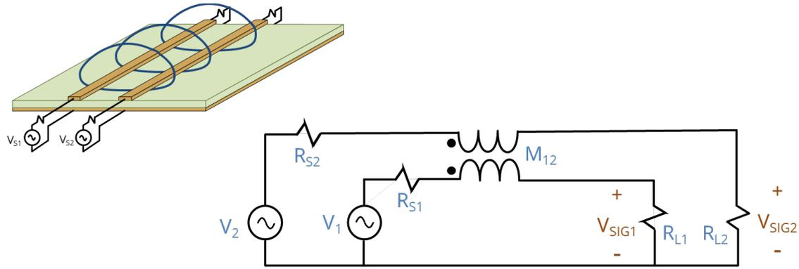
**Figure 6.4.** Schematic representation of magnetic-field coupling between traces.
