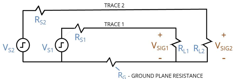
**Figure 6.2.** Schematic representation of traces with common return resistance.
