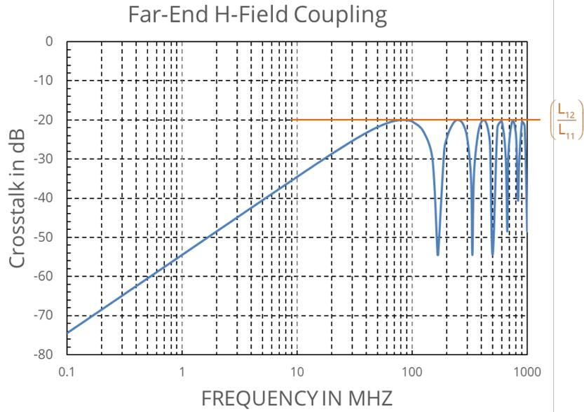
**Figure 6.9.** Far-end crosstalk between two matched transmission lines due to H-field coupling.
