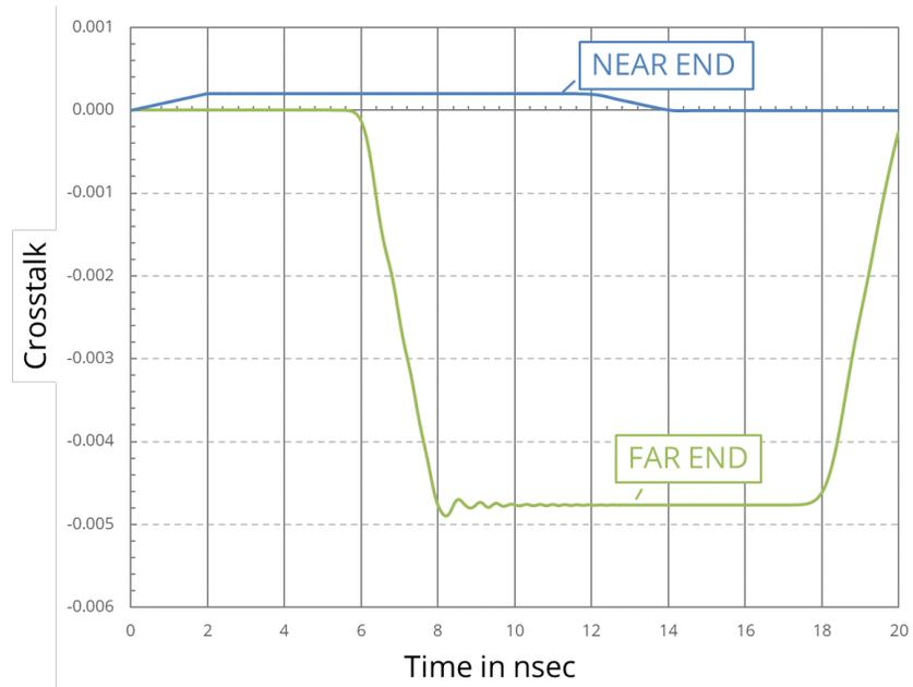
**Figure 6.24.** Calculated crosstalk with  $C_{12}/C_{22} = L_{12}/L_{11} = 10^{-2}$  and  $R_{NE2}=1 \Omega$ .
