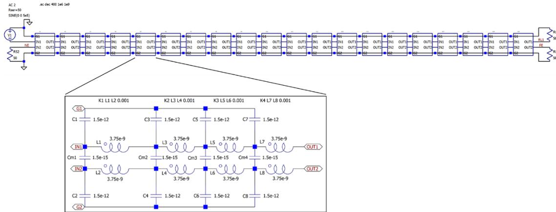
**Figure 6.16.** SPICE Model of coupled transmission lines with 80 LC sections.
