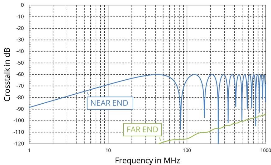
**Figure 6.17.** Calculated crosstalk between two lines with  $C_{12}/C_{22} = L_{12}/L_{11} = 10^{-3}$ .
