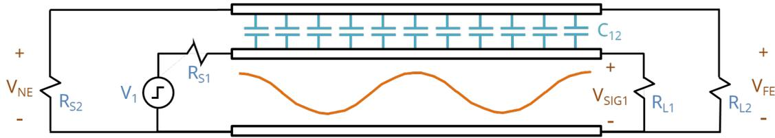
**Figure 6.6.** Lumped element model of electric field coupling.
