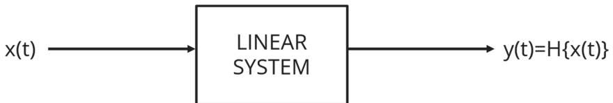
Figure 4.4. A linear system with input x(t) and output y(t) .
